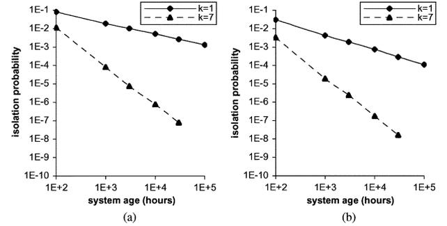
Fig. 8. Simulation results of  $\phi$  under age-proportional selection as system age  $\mathcal{T}$  and size  $n$  increase for Pareto lifetimes with  $E[L] = 0.5$  h. (a)  $\alpha = 1.5$ ,  $S = \infty$ . (b)  $\alpha = 1.2$ ,  $S = \infty$ .
