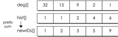
Fig. 8. Descending-degree relabel with a histogram.
