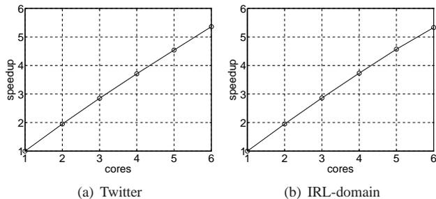
Fig. 9. Speedup vs. number of cores (8 GB of RAM).
