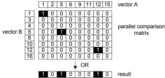
Fig. 7. Parallel intersection with STTNI.
