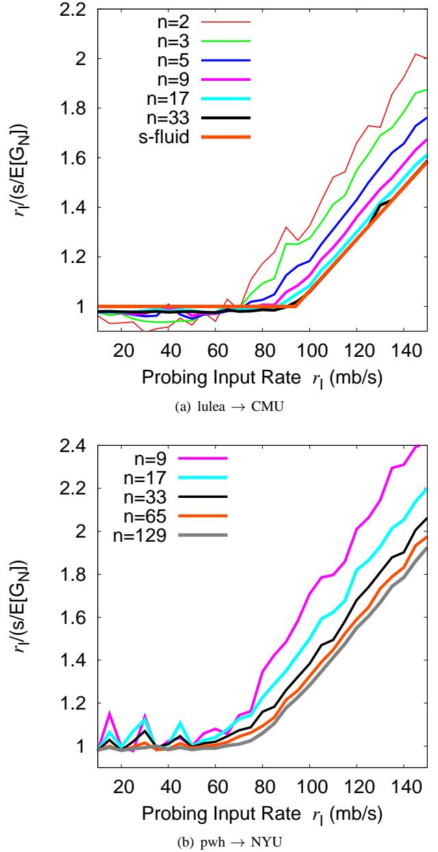
Fig. 4. Measured response curves of two Internet paths in RON testbed .
