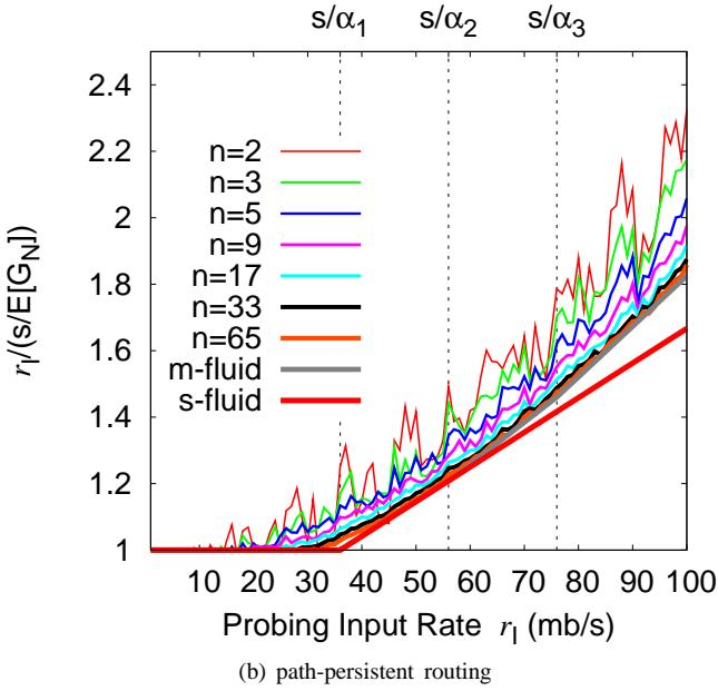
Fig. 2. Measured response curves using different packet train-length in the Emulab testbed.
