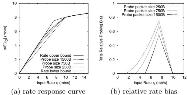
**Figure 5: Packet pair probing in CBR cross-traffic: (a) Rate response curves, (b) relative rate probing biases.  $C=10\text{mb/ps}$ ,  $\lambda=2.5\text{mb/ps}$ .**
