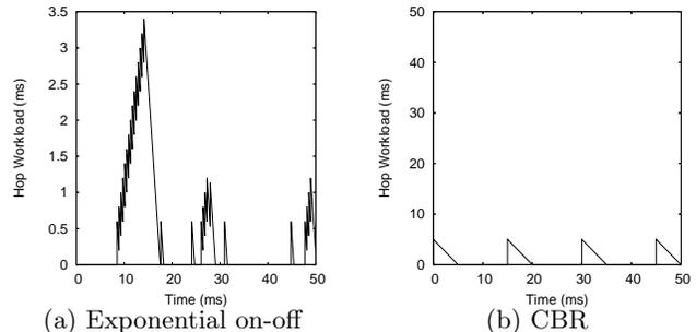
**Figure 2:** (a) The first 50 ms of the workload sample-path  $W(t)$  of exponential on-off ns2 traffic ( $C = 10$  mb/s,  $s = 750$  bytes); (b) Hop workload  $W(t)$  of CBR ns2 traffic ( $C = 2.4$  mb/s,  $s = 1500$  bytes).
