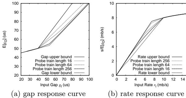
**Figure 6: Packet train probing in CBR traffic: (a) Gap response curves, and (b) rate response curves.  $C=10\text{mb/ps}$ ,  $\lambda=2.5\text{mb/ps}$ .**
