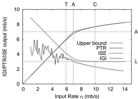
**Figure 12: Trace driven testing of three estimators: IGI, PTR, and ISE using PCS cross-traffic.**
