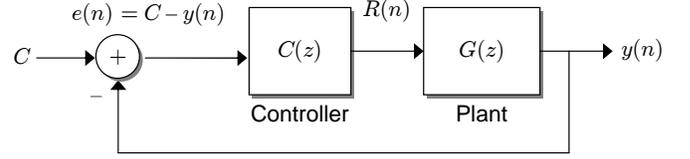
Fig. 7. Feedback control system model of explicit congestion control
