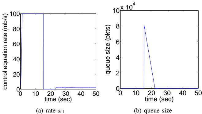
Fig. 3. Performance of RCP after abrupt increase in traffic demand at  $t = 15$ .
