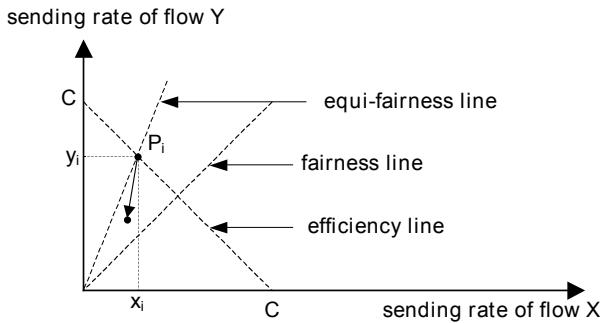
Figure 1. Two-flow I-D control system.
