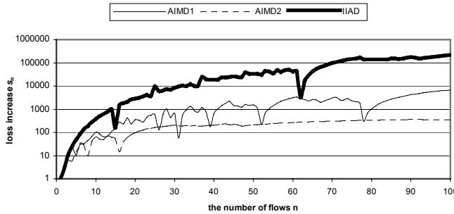
Figure 3. Parameter  $s_n$  (i.e., packet-loss scalability) of AIMD and IIAD in simulation based on actual packet loss.
