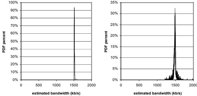
Figure 5. The PDFs of bandwidth estimates with 2 (left) and 32 (right) AIMD( $1,\frac{1}{2}$ ) flows over a shared T1 link.
