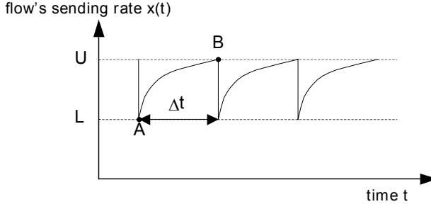
Figure 2. Oscillation of the sending rate in the stable state.
