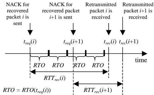
Figure 2. Operation of an RTO estimator given our trace data.
