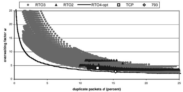
Figure 4. Performance of TCP-like estimators in ISP<sub>a</sub>.
