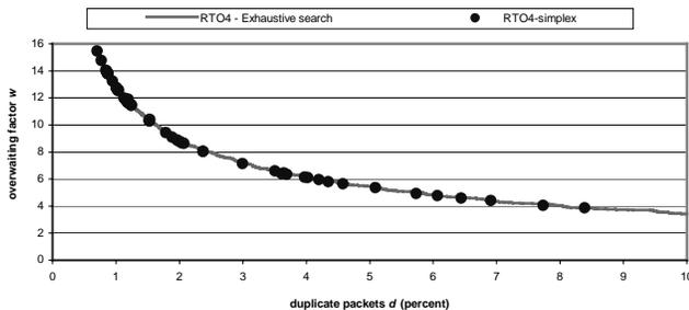
Figure 5. Points built by Downhill Simplex and the exhaustive search in the optimal  $RTO_4$  curve.
