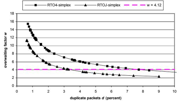
Figure 10. Jitter-based RTO estimators compared with the  $RTO_4$  estimator.
