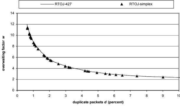
**Figure 11. Reduced jitter-based estimator compared with the optimal  $RTO_J$  estimator.**
