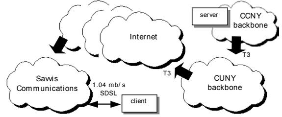
**Figure 12. The setup of the high-speed experiment.**
