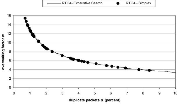
**Figure 7. Points built by Downhill Simplex and the exhaustive search in the optimal  $RTO_4$  curve.**
