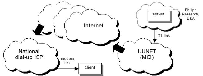
Figure 2. The setup of the modem experiment.
